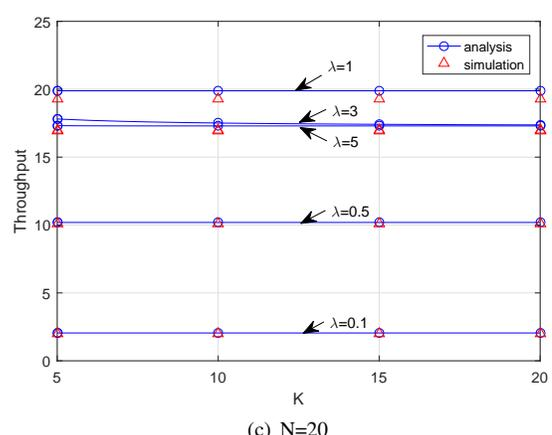
Fig. 4: Comparison of the system throughput varying  $R$  with different  $\lambda$  between analysis and simulation.
