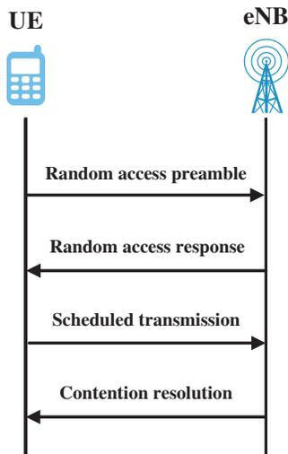
Fig. 1: Procedure of random access in NB-IoT.
