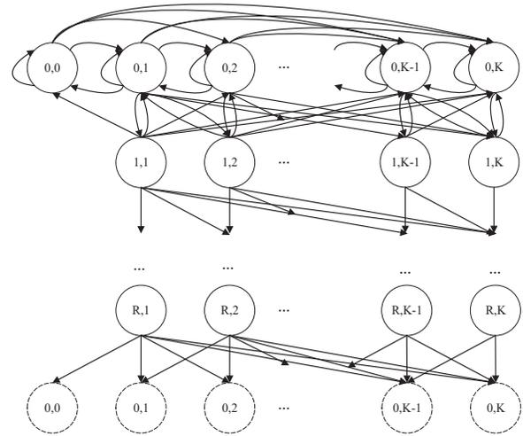
Fig. 2: The Markov chain for queue in NB-IoT.
